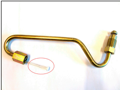
Oil pipe plus filter
