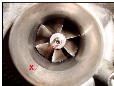
Missing lock nut
