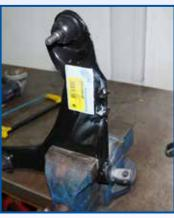
4. To protect against corrosion it is necessary to cover the exposed bare metal. Apply a layer of primer to the bare metal. Then once dry, apply a coating of an oil based paint. Alternatively use a good quality stone-chip guard type paint.
