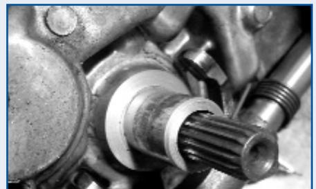
Transmission guide tube wear
