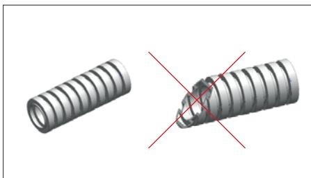
2. Insert the corresponding seal into the first groove of the corrugated pipe. The seal to be mounted on the vehicle side must be selected according to the corrugated pipe installed in the vehicle, because the corrugated pipe thicknesses may differ depend-
