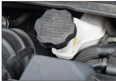
**Cause: Leaky cap on the brake fluid reservoir**
