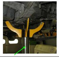
Use the appropriate device to assembly and disassembly the gearbox. The operator never must support the weight of gearbox.
