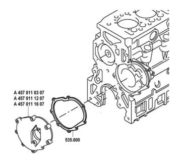
In order to improve seal performance between the camshaft sprocket cover and the engine block, a new Metaloseal<sup>®</sup> has been developed. It replaces the sealing compound that was previously used for this joint.
