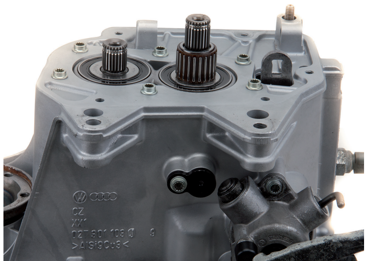
Twin-bearing mounting plate assembly and needle bearings of a 02T transmission
