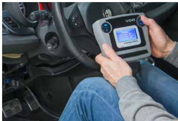
Basic adjustment with a suitable diagnostic tool
