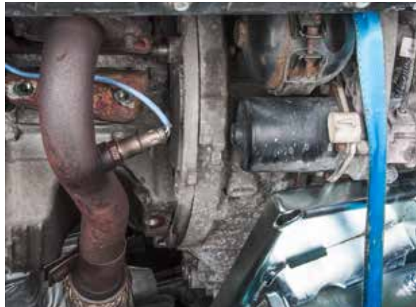
Bring the transmission as close as possible to the engine
