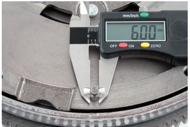
Fig. 1: Measuring the diameter of the clutch dowel
