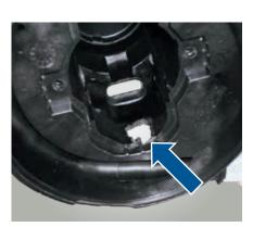
Damage: melting traces on the housing (top view into the housing)
