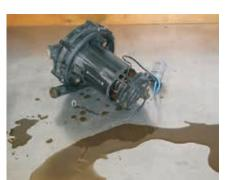
Liquid exhaust gas condensate from a secondary-air pump
