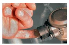
Finger check at secondary-air valve in BMW 520i (highlighted) If deposits are found on this end, the non-return valve is leaking and must be replaced.
