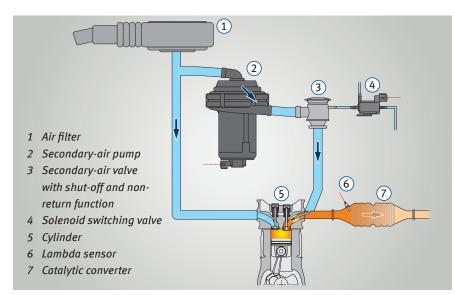
Block diagram of secondary-air system (pneumatically actuated)
