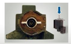
Corroded solenoid switching valve (open)
