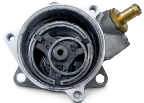
*Lack of lubrication oil due to old or contaminated engine oil.*
