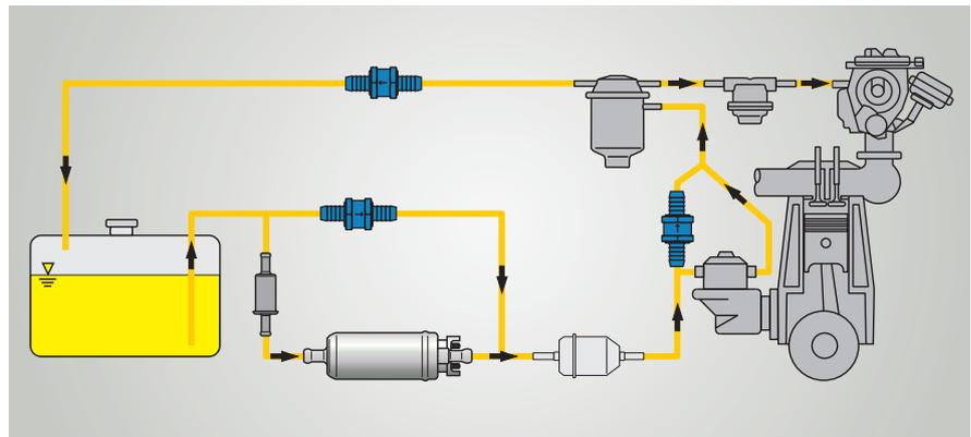
Application example: Carburettor engine with connectible supplementary electrical pump
