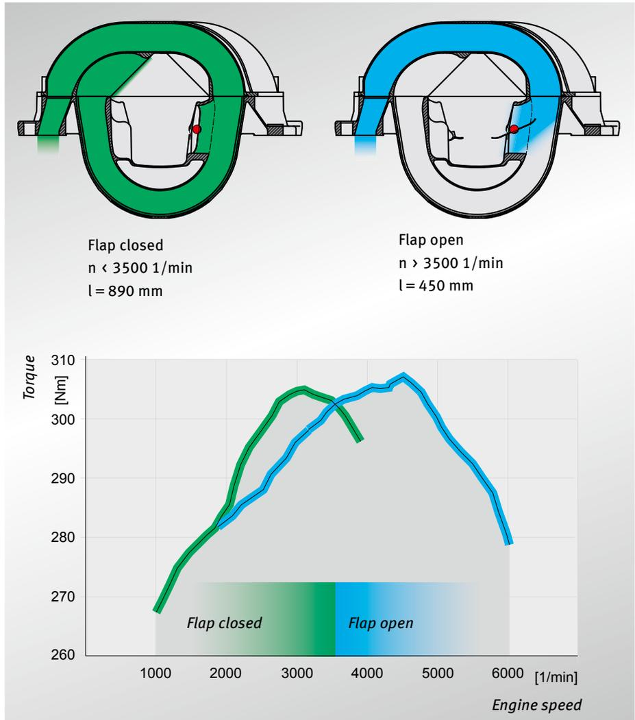
Example: Variable intake manifold in Mercedes-Benz V6 3.2l engine
