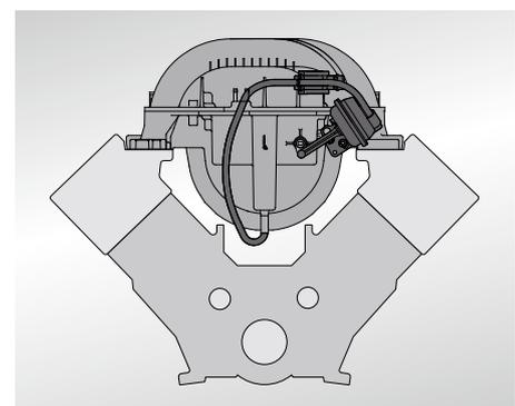
*Variable intake manifold on a V engine*
