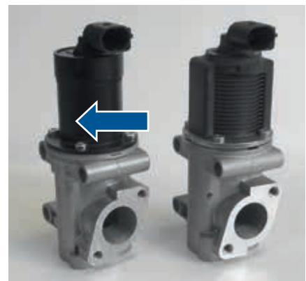
Image 5: Original coil body was replaced by simple turned part (arrow).
