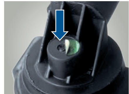
Image 2: This bore (arrow) can lead to water penetration and failure.
