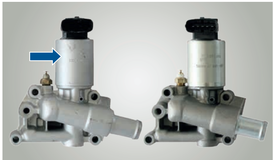
Image 1: A painted EGR valve (arrow) looks like new – but it is not.
