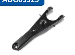
We have found that the cause of the problem can lie with a crack in the clutch release fork, as the release fork on this model can fracture and flex during operation and not allow the clutch to fully disengage.
