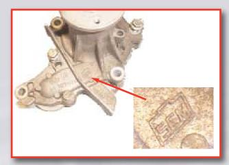
The original SEM type pump can be identified by the manufacturer's mark on the outer casing (see picture)
