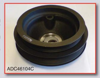
If the Crankshaft pulley is operating with a worn rubber damper at high engine RPM, the pulley can oscillate and in extreme cases there is a possibility that the outer part of the pulley can come adrift.
