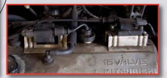
Blue Print strongly recommend that the spark plugs and HT leads are replaced in addition to the coil assembly, or that they are carefully checked. We also recommend that a logical diagnosis procedure is followed (prior to replacing the ignition coil) to prevent it being replaced unnecessarily.
