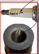
**Example B** shows where the spark has tracked along the spark plug ceramic (see burn marks).
