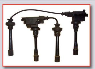
or high resistances in the spark plug or HT leads. Tracking can sometimes be visible or audible during operation, and may leave carbon traces where regular tracking to earth is occurring.
