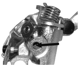
Wind the 4 mm hexagon screw clockwise until the brake pads pads touch the brake disc.
