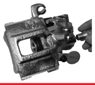
Wind back anti-clockwise until the disc can be turned freely.
