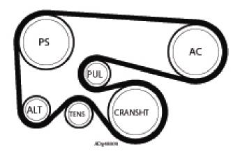
This means that the 6PK1840, previously recommended for some of these applications, should no longer be installed on this 1.9 JTD + AC drive. For correct actual applications, please check our online catalogue.
