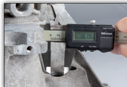
Image 2: If the diameter is smaller than 21 mm, it must be bored open to at least 21 mm, with a max. of 24 mm
