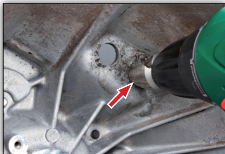
Image 5: Increasing the size of the holes
