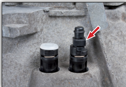
Image 8: The vent nipple can be actuated by hand or with a spanner (SW 13)
