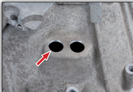
Image 6: Deburring and cleaning
